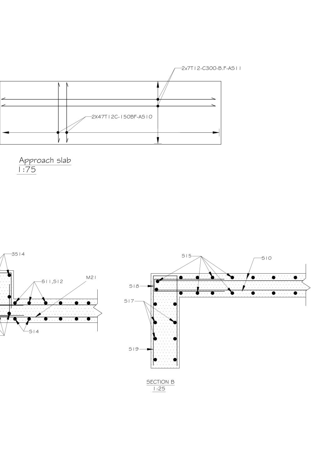
2] The following bars may be lapped[lap length at least 50times bar dia.: S10 and S20 the joints shall be well staggered
