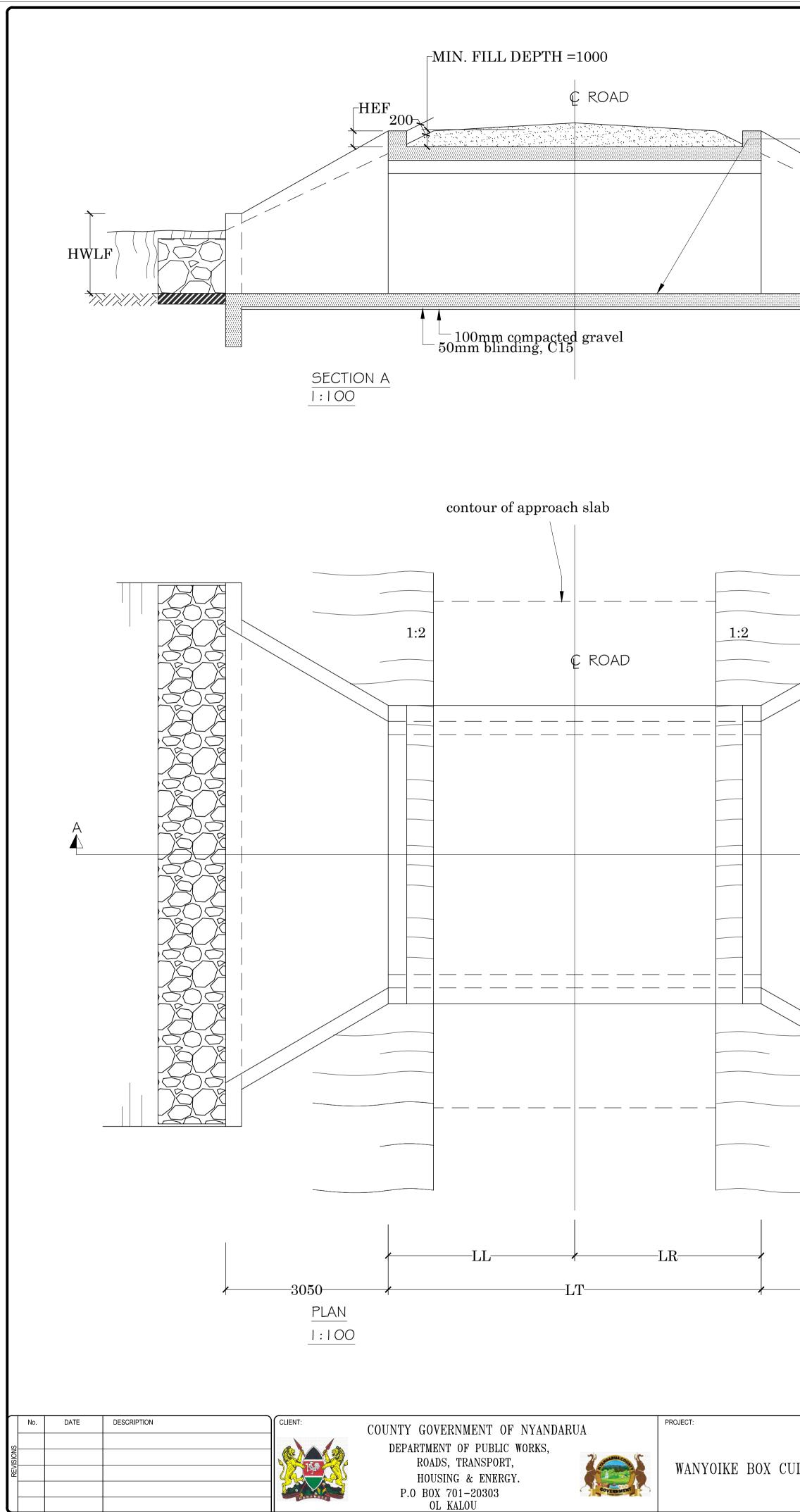
Bottom of culvert to be in line with existing river bed. Direction of flow, see plan and proflie drawing
